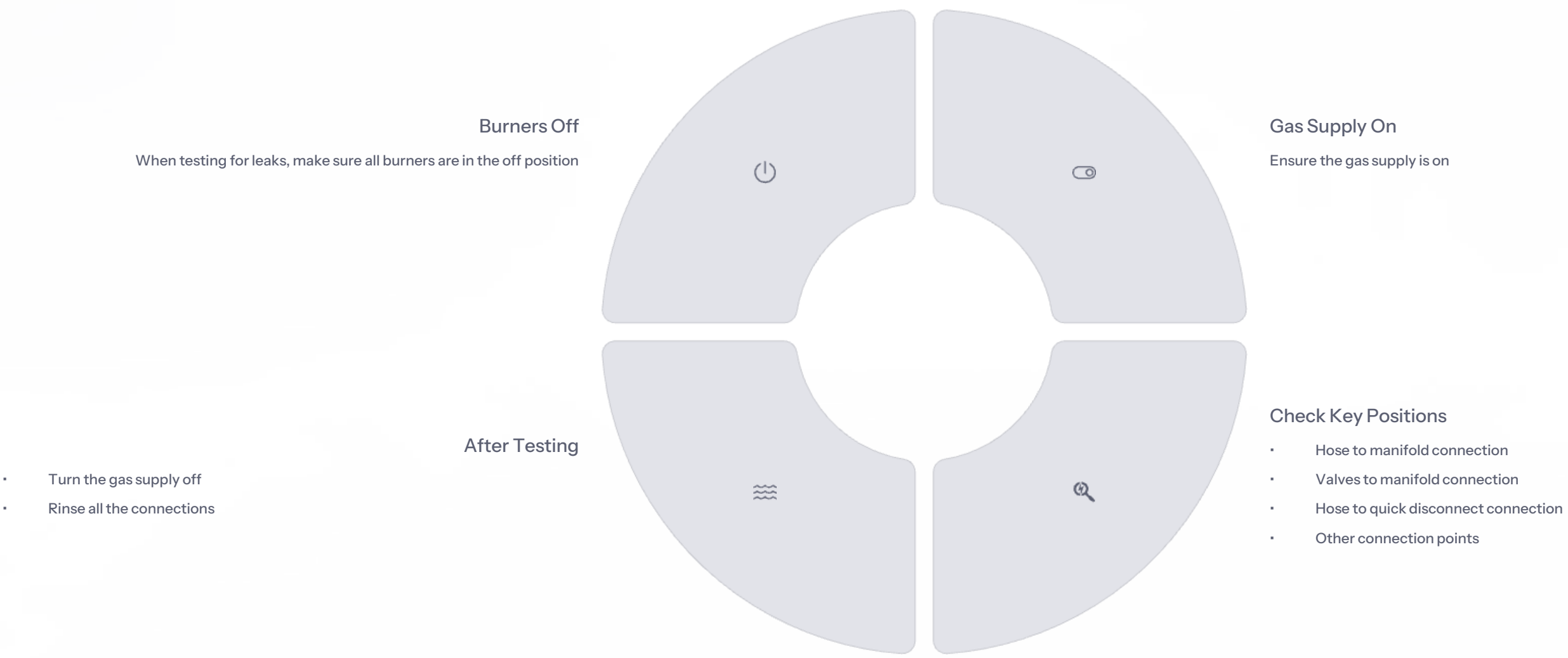
Figure 3-4 Gas leak checks
